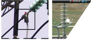
HD corona camera with features that boost corona detection and visualization. LuminarHD is the optimal choice when asking to streamline monitoring tasks. Outstanding optics and sensitivity to UV ensure unparalleled performance and clear display of pinpointed corona from far away and nearby. High definition recording lets users see more when analyzing the recorded media.
