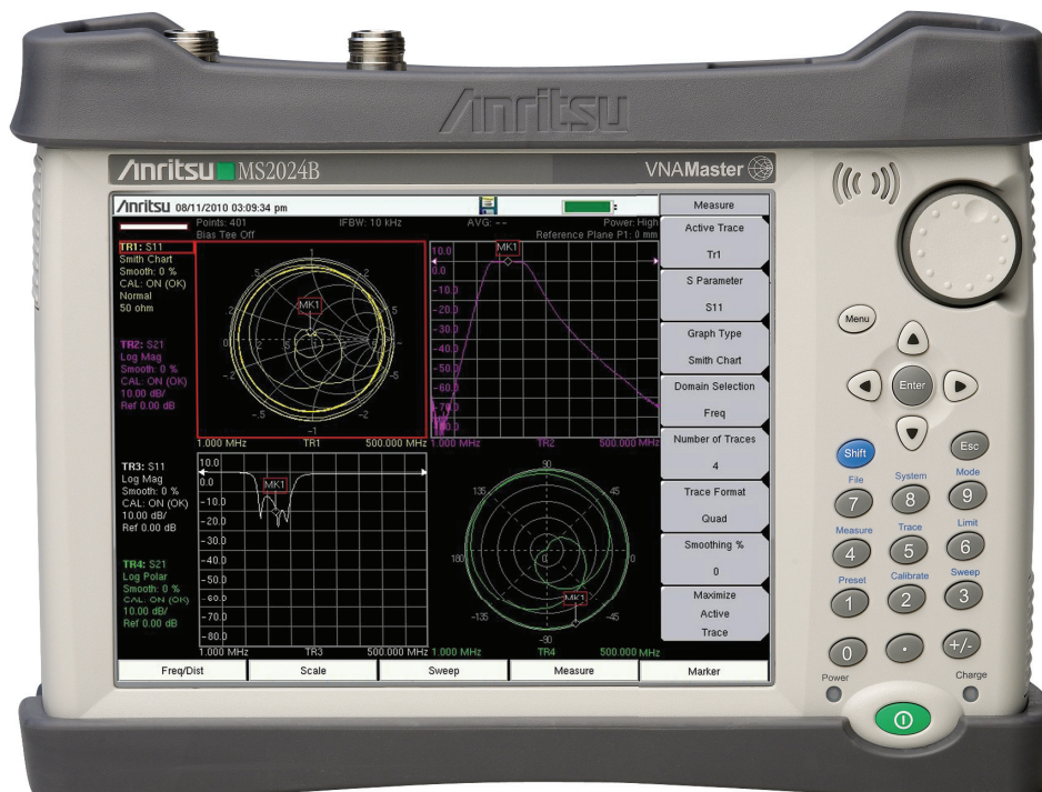
Size: Width - 273 mm (10.7 in), Height - 199 mm (7.8 in), Depth - 91 mm (3.6 in). Weight: 3.5 kg (7.6 lb).
