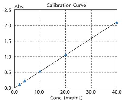
Note: One method of determining the lower limit of quantitation is to use ten times the standard deviation. This is an actual measured value and is not guaranteed.
