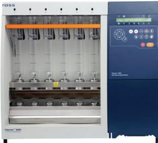
Fibertec™ 8000 is a fully automated system for determination of crude fibre, detergent fibre and related parameters according to standard reference 'crucible' methods such as Weende, van Soest etc.
