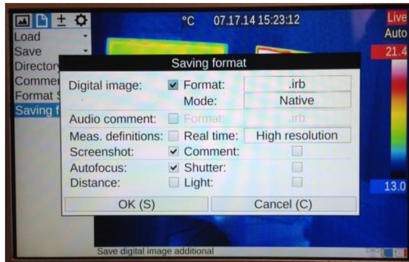
Select saving format including format, audio comment, level of resolution, comments, etc.
