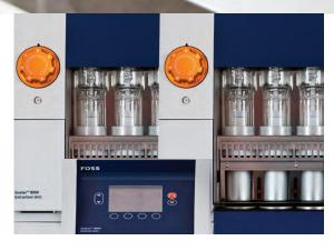
Operate two solvent extraction units from one control unit for reduced manual handling.
