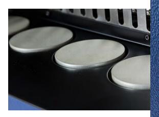
Hotplates with individual temperature control and automatic shutdown feature that allows out-of-hours operation.
