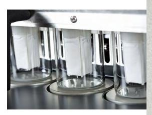
The unique, patented Hydrocap filter contains the sample all the way from initial weighing through hydrolysis to final extraction.
