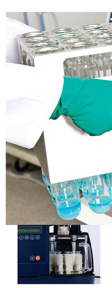
12-place hydrolysis sample holder for unattended operation and higher throughput.
