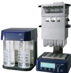
Tecator™ Digestion systems, with integrated programmable controllers, provide economical and efficient digestion for Kjeldahl analysis. A digestion system is based on a digestion block and tube rack with capacity for either eight, twenty or forty tubes.
