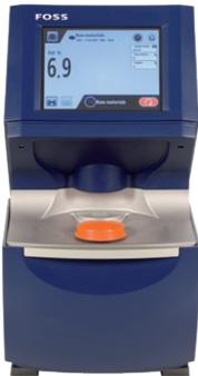
MeatScan™ measures fat in raw meat and meat products. It can be used by anyone and placed anywhere in the production for checking incoming raw material, control standardisation of batches, check fat content in final products etc. The analyser is particularly relevant and dedicated for small and medium sized plants. The analyser can be networked for remote access and support. For more advanced requirements, the FoodScan™ 2 is an ideal upgrade option.
