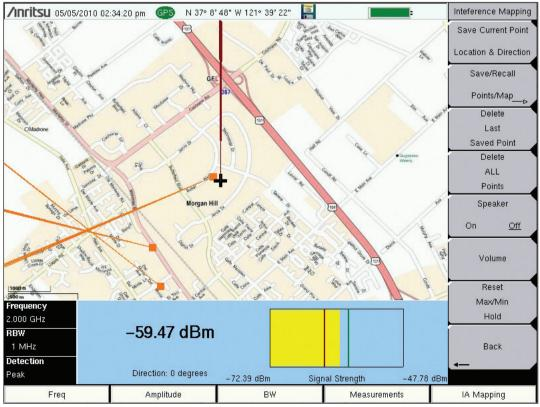
On Screen Interference Mapping
