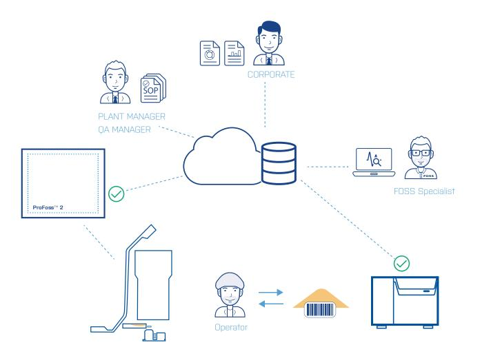
Software and digital connectivity services contribute to reliable performance across individual or whole populations of instruments. ProFoss 2 units can be monitored and managed from a single desktop, for example, when making calibration adjustments or proactively planning maintenance cycles for optimal uptime. This can be done from anywhere in the world from any PC.
