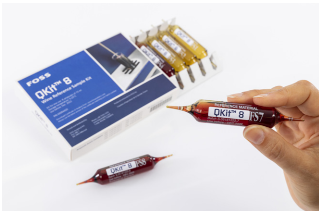
The QKit 8 is a set of eight wine samples with certified reference data on selected applications.
