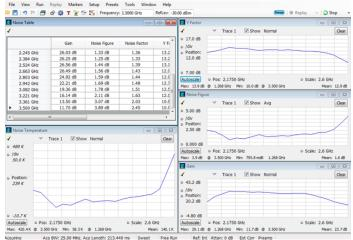
Noise Figure and Gain measurements (Option 14) help you to quickly and easily measure your device using the RTSA and a noise source. This image shows the measurement summary table with graphs of noise temperature, gain, noise figure and Y-factor.
