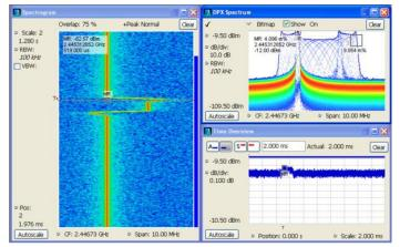
Trigger and Capture: The DPX Density<sup>™</sup> Trigger monitors for changes in the frequency domain, and captures any violations into memory. The spectrogram display (left panel) shows frequency and amplitude changing over time. By selecting the point in time in the spectrogram where the spectrum violation triggered the DPX Density<sup>™</sup> Trigger, the frequency domain view (right panel) automatically updates to show the detailed spectrum view at that precise moment in time.
