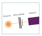
1. Infrared light through sample 2 Spectrum analysis
