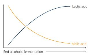
Rapid analysis allows you to track conversion of malic acid to lactic acid with a simple convenient test
